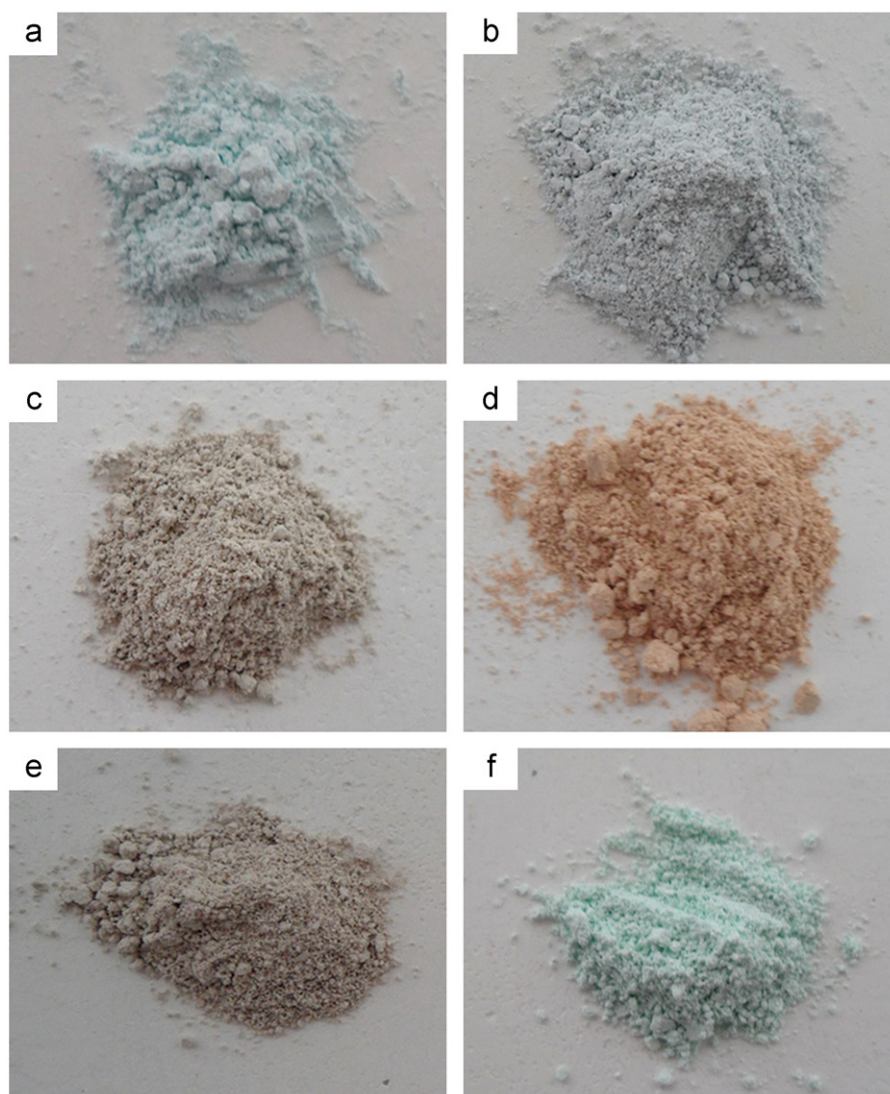
Fig. 3. Appearance of intermediate product at different temperatures and times: in heating process (a) 840 °C; in constant temperature process at 870 °C for (b) 30 min, (c) 120 min, (d) 240 min; in cooling process (e) 600 °C, (f) 500 °C. (For interpretation of the references to color in this figure caption, the reader is referred to the web version of this article.)
